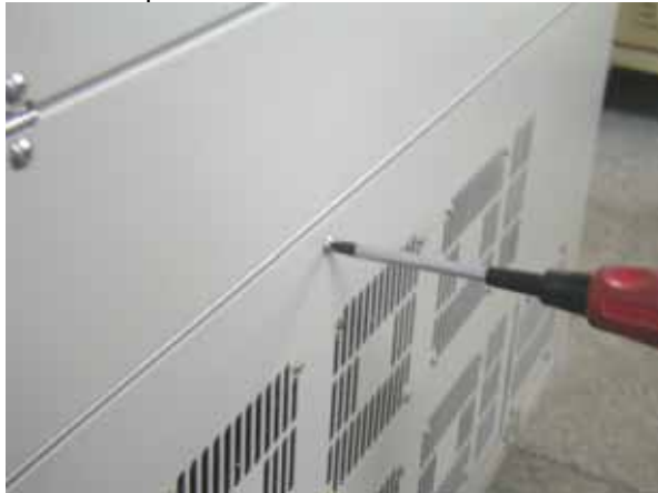
Fig. 4-2 Unscrew the Laser Cabinet
