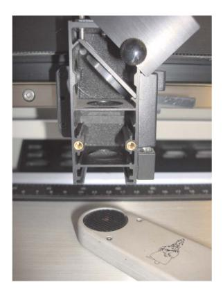
Place the **Black Target** of the power meter below the lens carriage so that the red dot is in the center. You do not have to be very accurate as far a center goes and focus does not mater as there is no lens.
